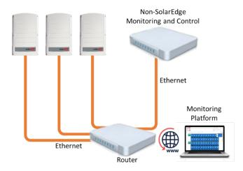
Option 2 – Connect the Leader only to the Ethernet router via Ethernet cables.
