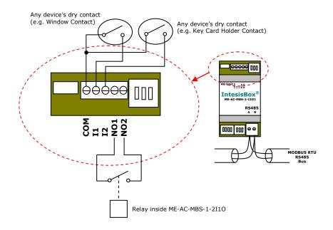
The relay output is also a dry contact normally open that can actuate any device with the following restrictions: 30VDC/5A, or 250VAC/5A max.
